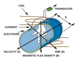
$E = K \times B \times V \times D$ K is instrument constant B is magnetic flex density V is average fluid velocity across the pipe D is diameter of measurement pipe
